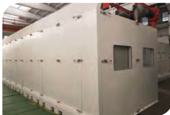
After Alternation: 4,000 rpm with noise reduction of more than 14dB in each district.
